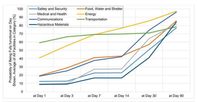
Figure 9-19. Critical Facility Functionality, Hayward Fault Scenario
