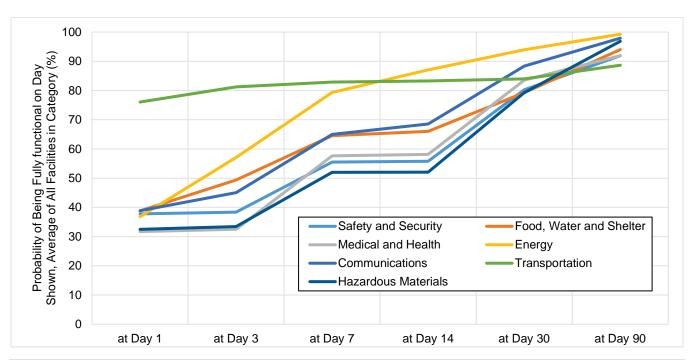
Figure 9-20. Critical Facility Functionality, Maacama Fault Scenario
