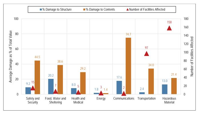
Figure 10-7. Estimated Damage to Critical Facilities from 1% Annual Chance Flood
