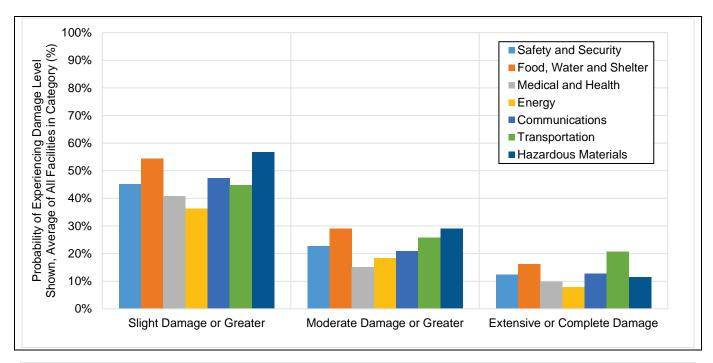
Figure 9-17. Critical Facility Damage Potential, San Andreas Scenario
