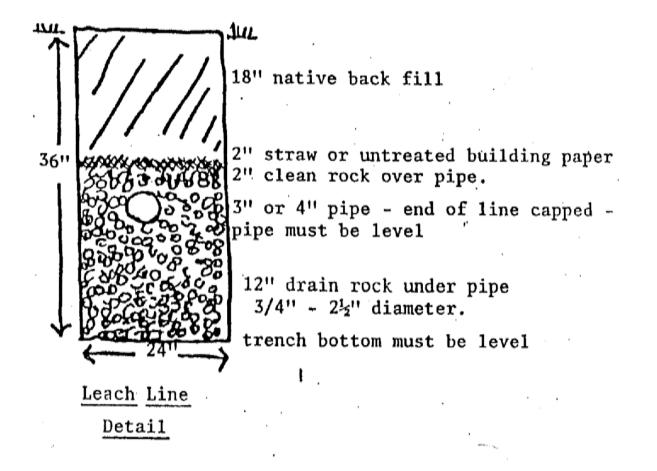
Note: Depth of trench dependent on slope and/or depth of rock below pipe. 30" deep system with 12" of drain rock under the pipe requires 12" of native backfill. Allowable width of standard leachline trench 18 - 24"
