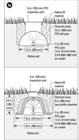
Cross sections of typical half-pipe and low-profile SPDS installations showing dimensions and materials
